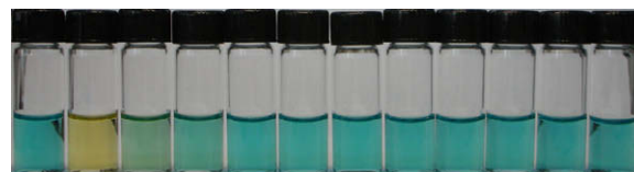
Figure 3. Color changes of ensemble 1 ( [\mathbf{1}] = 2.1 \times 10^{-5} M) in a 10 mM HEPES buffer (pH 7.4) at 25 °C after the addition of various anions (2 equiv, sodium salts). From left to right: Ensemble 1 , PPI, ATP, ADP, AMP, Pi, \text{AcO}^- , \text{NO}_3^- , \text{I}^- , \text{Br}^- , \text{Cl}^- , \text{F}^- .
